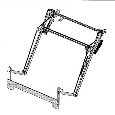
A series of sprockets located in the sweep drive channel carry the sweep chain between them. The sweep is powered by the main motor. The power generated by the motor is relayed to the sweep chain through the two sweep timing belts, with the second one being activated by a magnetic clutch when necessary.
