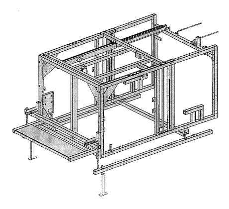
The frame provides the main support in suspending the pinsetter above the lane and pit. Screwed to the top of each kickback is the kickback tubing. The kickback tubing runs the entire length of the kickback and beyond in order to line up with the front of the pinsetter.
