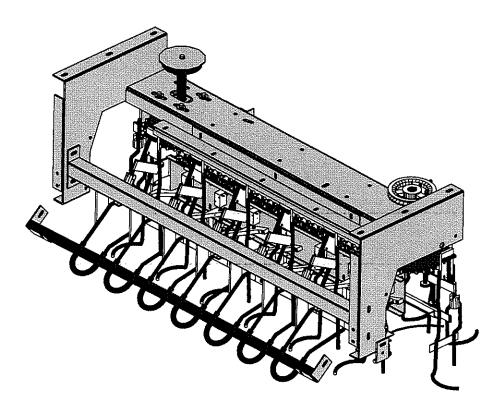
The continuous moving carrousel uses fourteen (14) pin loaders with permanent magnets to pick off the pins from the staging position. Each pin loader may pick up from the left or the right staging position and an empty pin loader will always pick off a pin if one is present in the carrousel staging.
