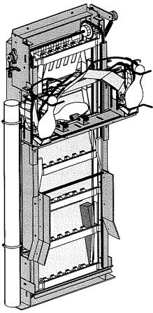
The pin elevator receives the pins from the pit conveyor belt and carries them up to the carrousel staging position using the elevator lifts. A series of sprockets located inside the left and right plates carry the elevator chains between them. The elevator is powered by the main motor. The power generated by the motor is relayed to the elevator chain through the stock timing belt and the elevator belt which is activated by a magnetic clutch when necessary.
