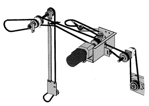
Located on the top of each pinsetter is the ½ hp main motor. Using a series of magnetic clutches, belts and pulleys, the main motor supplies the driving power to the sweep, the carrousel, the pin elevator and the pit.
