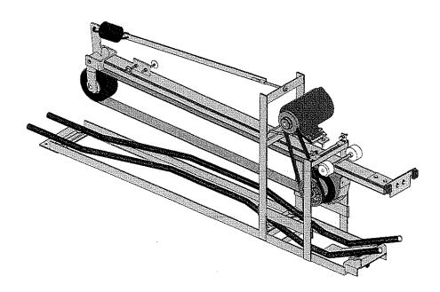
Fastened to the floor between each pair of pinsetters is the ball accelerator assembly which propels the ball to the ball return rack located at the bowler's end of the lane. Mounted on the accelerator's frame are two carriage bolts which exert pressure on both kickbacks in order to keep the accelerator belt and accelerator track parallel to each other.
