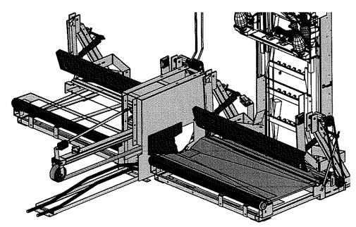
Located at the rear of each lane's pin deck is the pit which uses a conveyor belt to transport the deadwood to the pin elevator and the ball to the ball accelerator door. The conveyor belt travels on the front roller and the rear roller. The power generated by the main motor is continuously relayed to the rear rollers through the stock timing belt and the pit belt.
